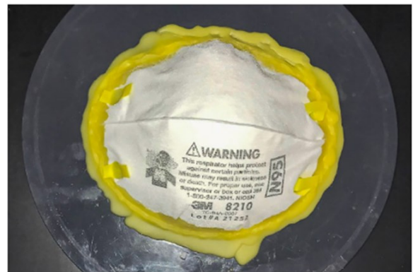
A N95 mask is tested in an ECU laboratory to validate effectiveness in preventing transmission of respiratory contaminants.
